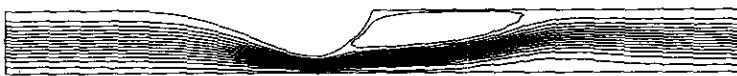
Figure 8. The streamline contours of the flow at Re = 100 , T^* = T_0^*/107 , P_d^* = P_{d0}^* . A flow separation is developed downstream. Contour interval is 0.075.
