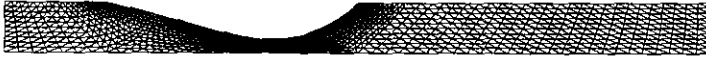
Figure 2. The finite element mesh of the flow domain (mesh-3), with 1642 6-node triangular elements and 3261 nodes.
