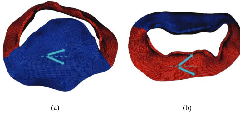
FIG. 3. Two families of fibre directions shown by arrows on anterior, shown in (a) (blue online) and posterior, shown in (b) (red online) leaflet. Circumferential direction is shown by the dashed line.
