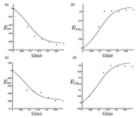
Figure 9. Strain comparisons between the BSDIR method (circle) and FE model (solid line) (a)  $E_{rr}$  in sector A, (b)  $E_{zz}$  in sector A, (c)  $E_{rr}$  in sector B, (d)  $E_{zz}$  in sector B in a long axis slice, Sectors A and B are zones near the midventricle. Overall, there is good agreement between the BSDIR method and numerical strains in sectors A and B.
