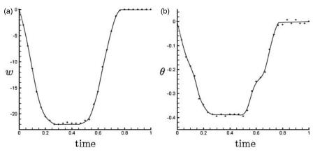
Figure 3. The motion of the apex plane for case A. The symbol (+) indicates the raw data obtained from camera recordings, fitted with splines. (a) Displacements (mm) in the long axis direction versus time (s), and (b) rotational angle  $\theta$  (radian) versus time (s).
