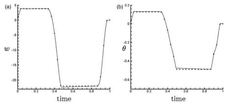
Figure 4. The motion of the apex plane for case B. The symbol (+) indicates the raw data obtained from camera recordings, fitted with splines. (a) Displacements (mm) in the long axis direction versus time (s), and (b) rotational angle  $\theta$  (radian) versus time (s).
