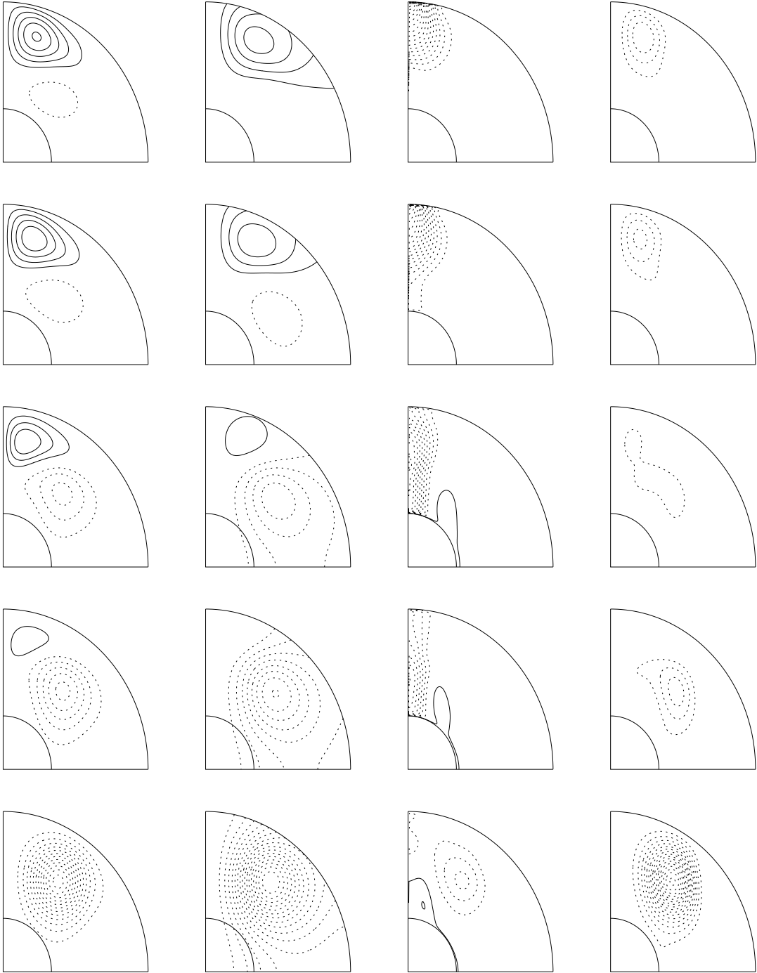
Figure 6: Contour plots of the field B (1st column), Ar \sin \theta (2nd column), the flow v/r \sin \theta (3rd column) and \psi r \sin \theta (4th column) at five times: t_0, t_0 + 0.4, t_0 + 0.8, t_0 + 0.9, t_0 + 1.0 (top to bottom) for \alpha_0 = 11 and E = 2.5 \times 10^{-4} . The corresponding magnetic energies are E_M = 4.80, 4.26, 4.68, 8.80 and 41.0 . The minimum of E_M \approx 3.99 is at about t_0 + 0.62 . Contour intervals are 0.5, 0.05, 10 and 0.1 respectively. Solid lines represent positive and dashed lines represent negative contours.
