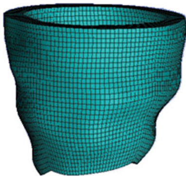
Fig. 6 The “cylindrical region” of the LV, where residual stress is considered. Residual stresses are not included near the apex
