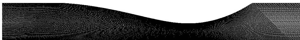
Fig. 4. A typical mesh for the deformed system in the Adina model.
