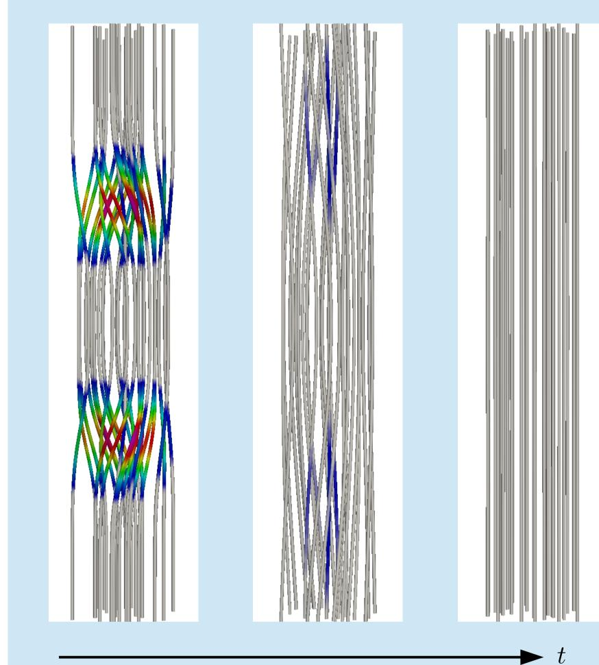
Evolution of the magnetic streamlines for a simply braided magnetic field. As expected, the field relaxes into the potential field with constant z-component.
