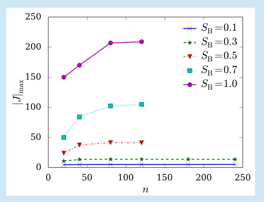
Maximum electric current density after relaxation for the sheared field configuration for different resolutions n and shearing strength  $S_{R}$ .
