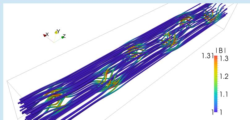
Initial magnetic field for the sheared field configuration. The colour coding shows the magnetic field strength.
