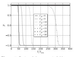
Figure 5. Parity of the magnetic field versus time for a random initial field in 3-D DNS.
