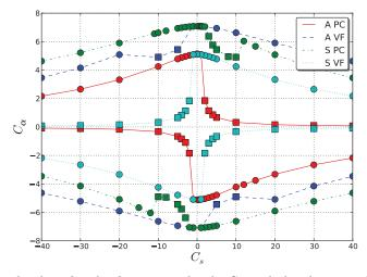
Figure 2. Critical values for the forcing amplitude  $C_{\alpha}$  and the shear amplitude  $C_{\rm s}$  for an  $\alpha\Omega$ -dynamo in 1-D mean-field to get excited. The circles denote oscillating solutions, while the squares denote stationary solutions.
