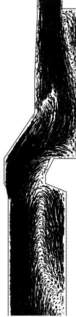
Figure 7.10: Flow through an idealised human upper airway. Velocity vectors
