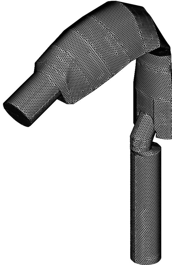
Figure 7.8: An idealised human upper airway model. Unstructured mesh.
