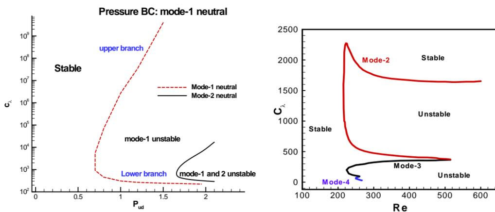
The cascade structure appears to be different for prescribed upstream pressure (left) and flow rate (right). Mode transition occurs when the wall stiffness is decreased.
