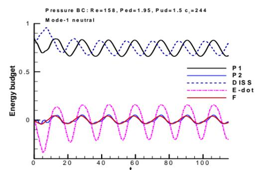
Energy budget shows that for mode-1 (pressure driven): rate of working of external pressure is most important, while for mode-2 (flow driven): rate of stretch energy change is dominant.
